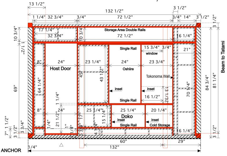
All 4x4 beams in the drawing project 1/4" beyond trailer bed Other woodwork and plywood siding is flush with edge of trailer bed.
