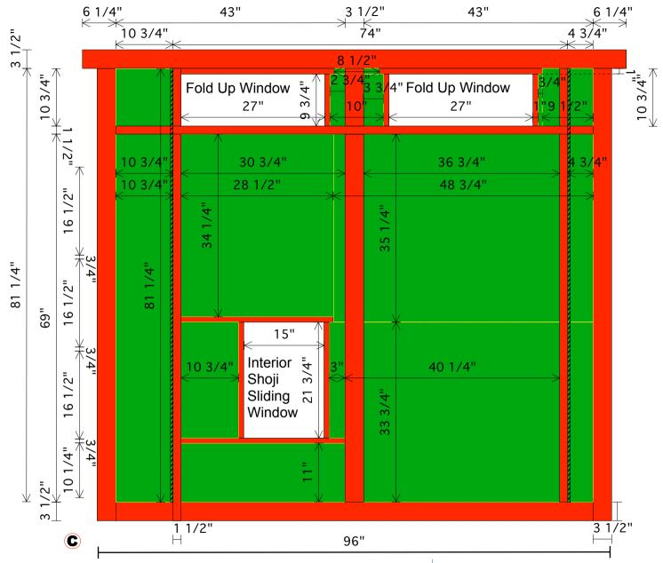
Note: Detail framing indicated in red is flush with the interior wall and uses 3/4" x 4 1/2" (1" x 5") Hinoki wood.
