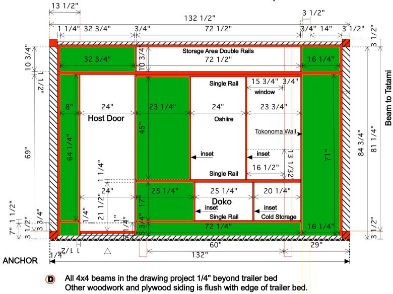
Use 3/4" x 5 1/2" (1 x 6) stock for the external frame for the window. This frame extends 2 1/2" beyond the interior surface of the plywood panel and 2 1/4" beyond the exterior surface of the plywood pannel. Use 3/4" x 3 1/2" (1 x 4) stock for the center divider. The divider extends to the outer surface of the plywood panel. Cut 28 3/4" x 20" hole frame for the window and insert plywood plug in the right hand half.
