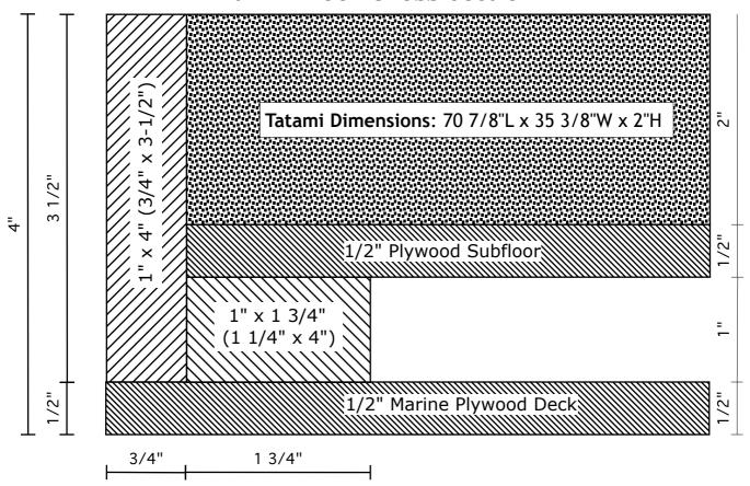
This design requires cork/rubber tape between the floor joists and the plywood subfloor to make up for the 1/32" deficit in the plywood.
